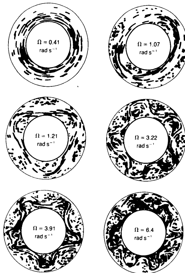
Fig. 15.10 Streak photographs revealing the flow in a series of rotating dishpan (annulus) experiments in which the rate of rotation was increased while the temperature gradient was held constant. Waves developed at higher rotation rates which became irregular for the highest rotation rates.
